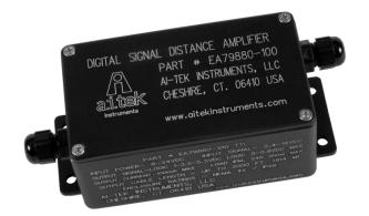
Line impedance plays a major role in the distance an active sensor signal can be transmitted through cable and wire. Mutual capacitance of 25 Pico-farads/foot or more can exist between conductors. When sufficient resistance from the sensor, cabling and output load is placed in series with that capacitance signal rise times can increase to the point where the sensor can no longer switch. This condition becomes even worse due to higher target speeds that cause output signal frequency rises
