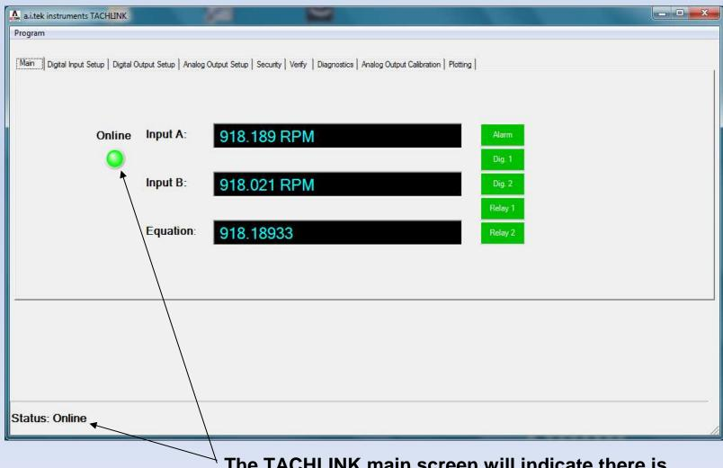
The TACHLINK main screen will indicate there is communication between PC and tachometer. (The "Online" light will be green and lit)
