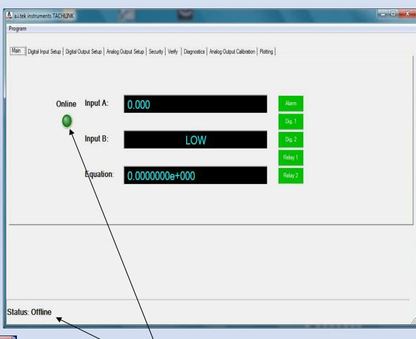
The TACHLINK main screen will also indicate there is no communication between PC and tachometer. (The "Online" light will be green but not lit)
