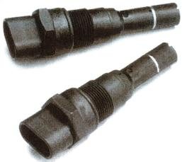
The new SLS uses a molded, glass filled nylon body to protect the sensor in harsh, truck-operating environments. It replaces the old fly-lead design with an integral standard Packard connector, which eliminates the added extra connector cost of the old design. It is available in single and dual output versions.
