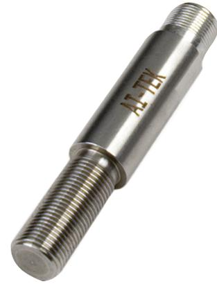
The new AI-TEK DH series sensors are differential based, zero-speed, precision, single channel, speed sensors. At power-up, they calibrate themselves to the unique magnetic signature of their installed application and continue to update the calibration as the sensor is running. This unique combination of differential sensing technology and calibration make these sensors highly tolerant of installation mis-alignment, target geometry and composition, target run-out, vibration and air gap changes.
