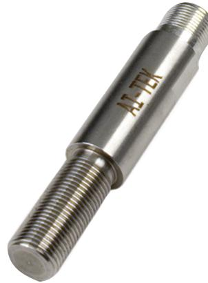
The new AI-TEK DH series sensors are differential based, zero-speed, precision, single channel, speed sensors. At power-up, they calibrate themselves to the unique magnetic signature of their installed application and continue to update the calibration as the sensor is running. This unique combination of differential sensing technology and calibration make these sensors highly tolerant of installation mis-alignment, target geometry and composition, target run-out, vibration and air gap changes.
