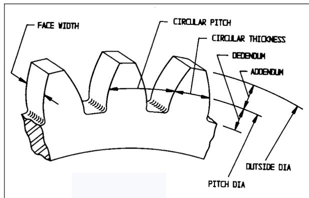
Figure 2 - Common terms used in defining gears.
