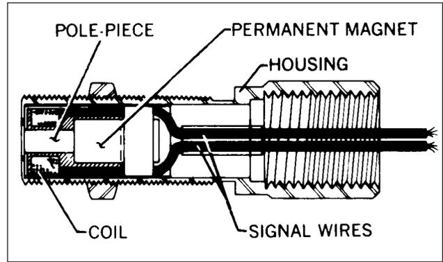
Figure 1 - Internal configuration of typical sensors.
